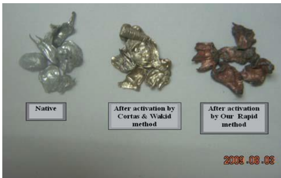
Figure 3.3: CuCd granules produced from both methods (Cortas et al., 1990)
